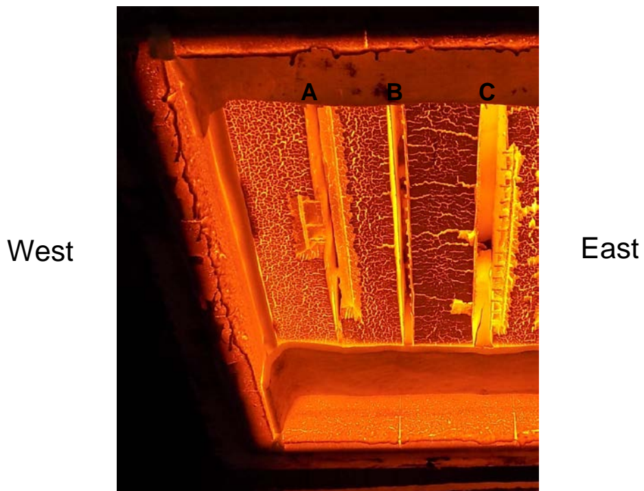
Figure A6.4: Exposed face of specimen at the end of the test.
