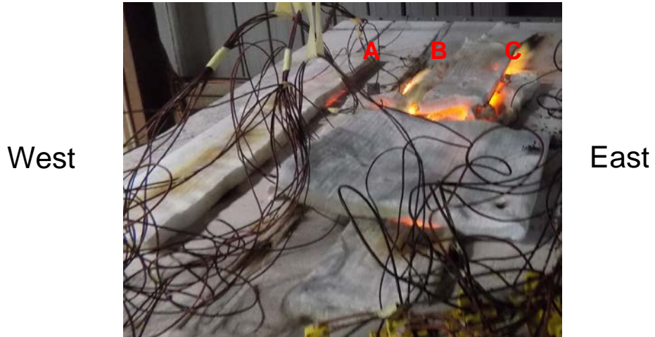
Figure A6.3: Unexposed face of specimen at the end of the test.
