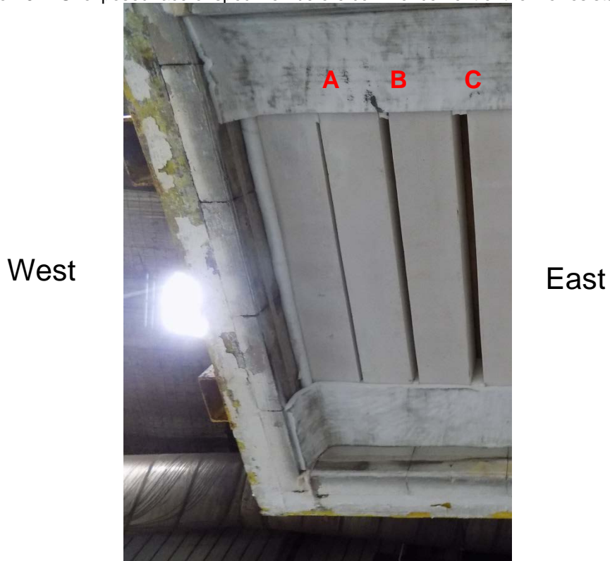
Figure A6.2: Exposed face of specimen before commencement of the fire-resistance test
