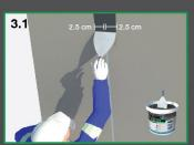
Apply RHINOZ Hybrid FX-55 along the joint To make surface smoother, can apply to fill the gap at thickness of 3-5 mm, and second layer of RHINOZ Hybrid FX-55 cover 2.5 cm width on both sides.
