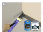
For wall/floor and wall/wall junctions and corners, after applying the 3D Elastic C200, while it is still wet, tape RHINOZ Fiberglass Mesh Tape over. Apply the second coat over the fiberglass, ensuring that all of the fiberglass is covered and let it dry.
