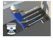
Apply the second coat of 3D Elastic C200 in crosswise direction to the first coat, allow it to completely dry for 7 days before tiling or filling water.
