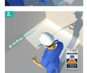
Apply 1 coat of **3D Primer Bonding** on the desired area, and apply it on boundary wall up to 10-20 cm above ground level. Let it dry for 30-60 minutes, or until it changes from milky white to clear.
